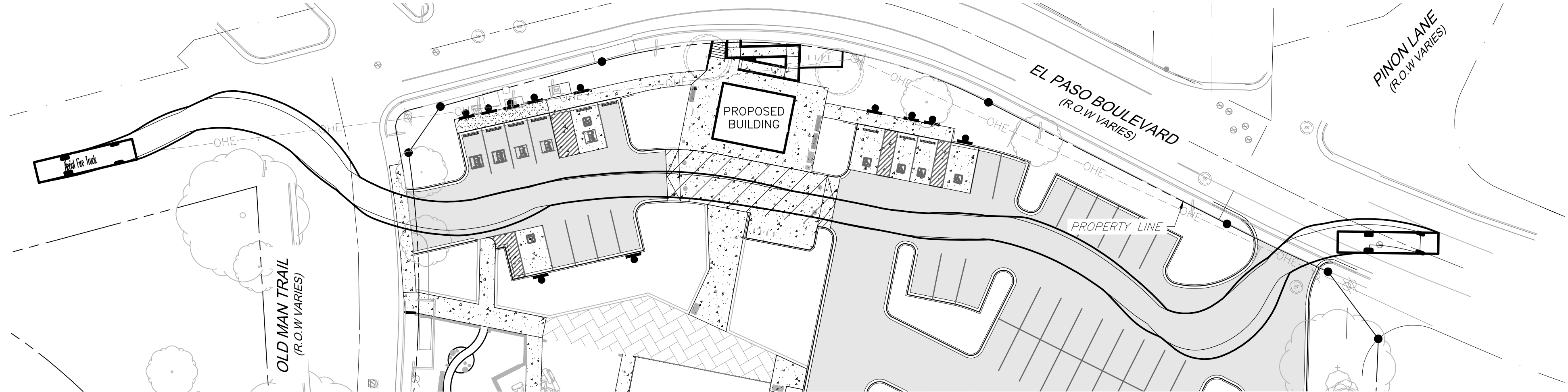
TRUCK TURNING TWO FIRE TRUCK
