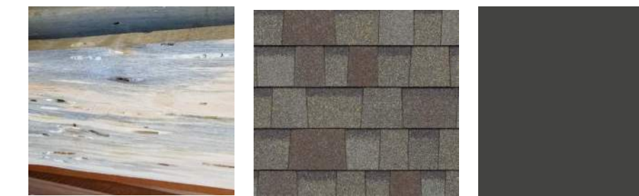
1x6 TONGUE AND GROOVE BEETLE KILL BLUE STAIN PINE RESTROOM SOFFIT TRUDEFINITION DURATION STORM SHINGLES - DRIFTWOOD SHERWIN-WILLIAMS SW 7069 IRON ORE METAL TRIM & RODS
