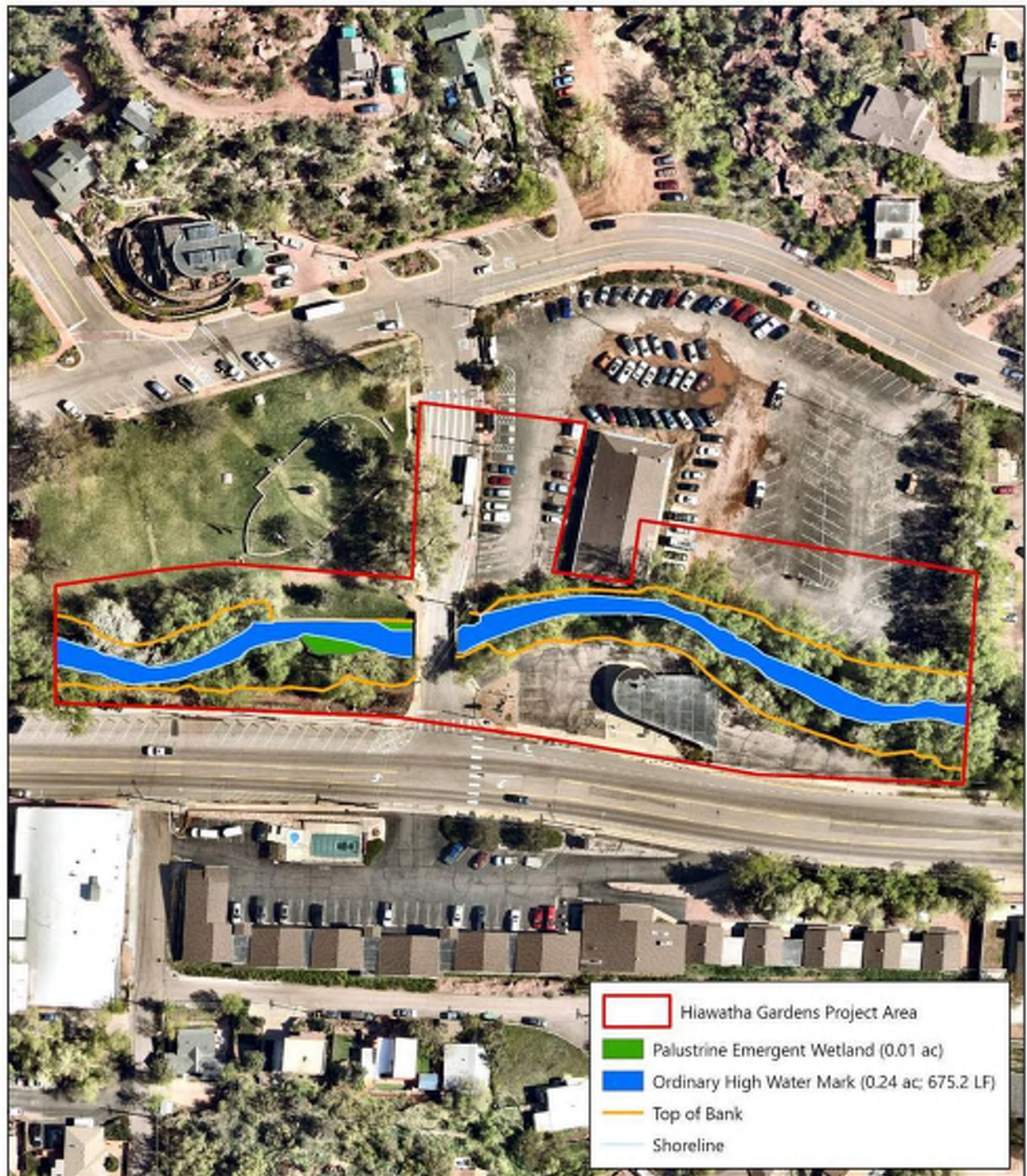
Figure 3. Ordinary High Water Mark, Top of Bank, and Shoreline
